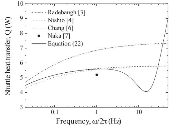
Fig. 5. Comparison of the current and existing expressions for shuttle heat transfer as a function of oscillating frequency.
