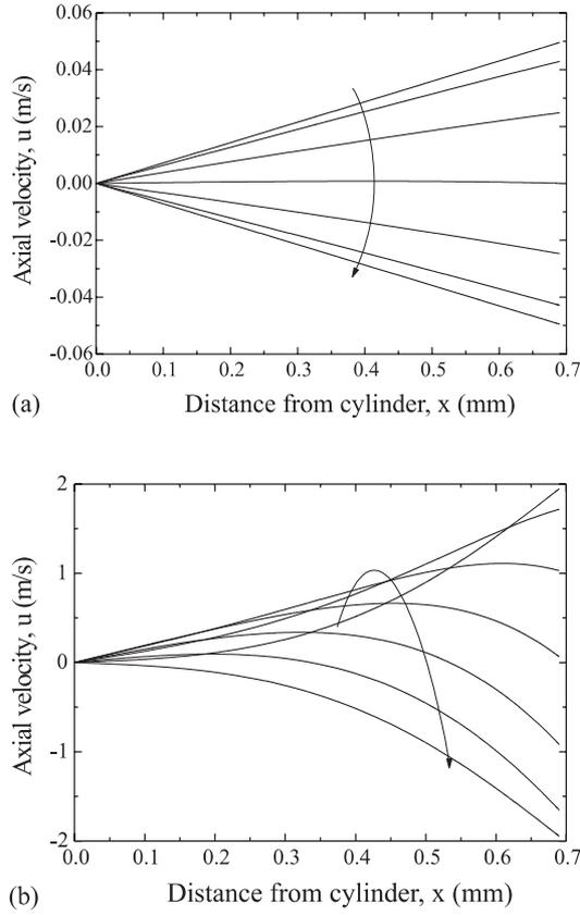
Fig. 3. Axial velocity profiles in  $\pi/6$  increments for half period: (a)  $\omega/2\pi = 0.5$  Hz, (b)  $\omega/2\pi = 20$  Hz.
