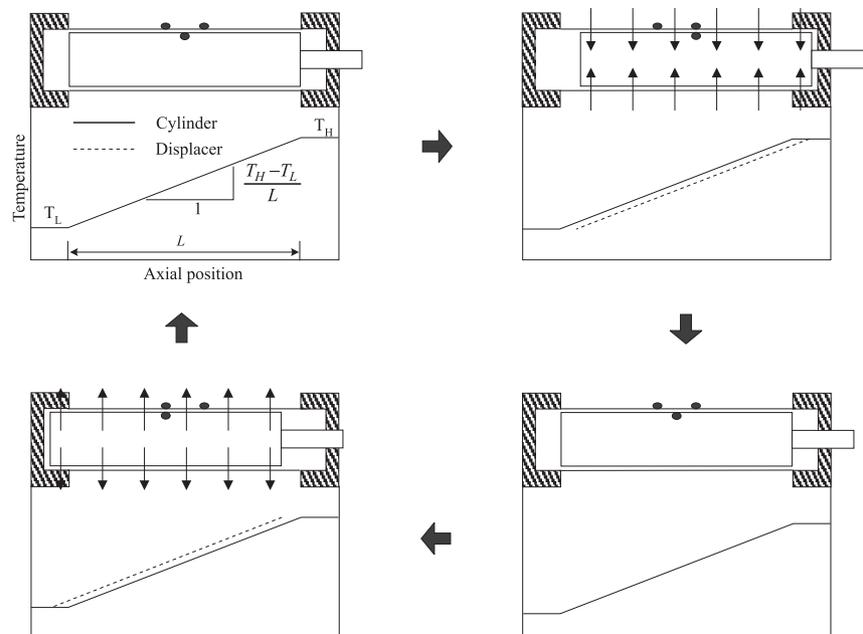
Fig. 1. Basic principle of shuttle heat transfer.
