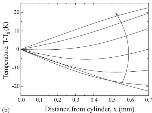
Fig. 4. Temperature profiles in  $\pi/6$  increments for half period: (a)  $\omega/2\pi = 0.5$  Hz, (b)  $\omega/2\pi = 20$  Hz.
