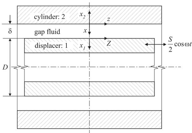
Fig. 2. Coordinates of displacer-cylinder system.
