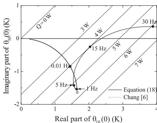
Fig. 6. Locus of complex temperature at displacer surface,  $\theta_{10}(0)$ , on complex plane at various frequencies.
