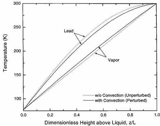
**FIGURE 2.** Vertical temperature distributions for the leads and vapor without (unperturbed) and with (perturbed) natural convection of vapor. ( $bL = 1.311$ ,  $h_l P/k_l = 0.000428$ ,  $k_l A_l/k_g A_g = 1.37$ )
