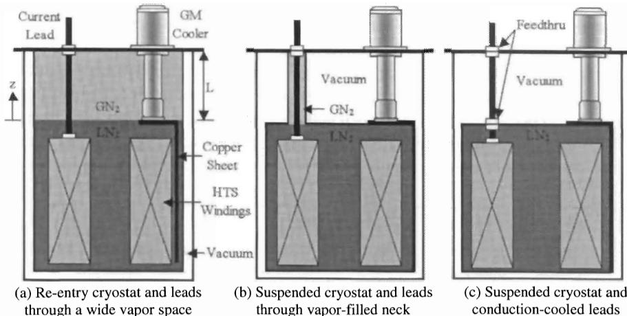
**FIGURE 1.** Schematic of three configurations of zero boil-off cryostat refrigerated by a cryocooler
