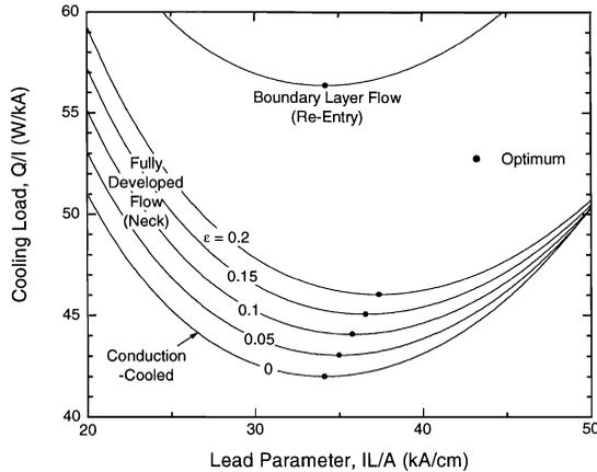
**FIGURE 3.** Cooling load of leads per unit current as a function of the lead parameter ( $IL/A$ ) for boundary layer flow and fully developed flow in comparison with conduction-cooled leads. (Copper with  $RRR = 60$ ,  $T_H = 300$  K,  $T_L = 77$  K)
