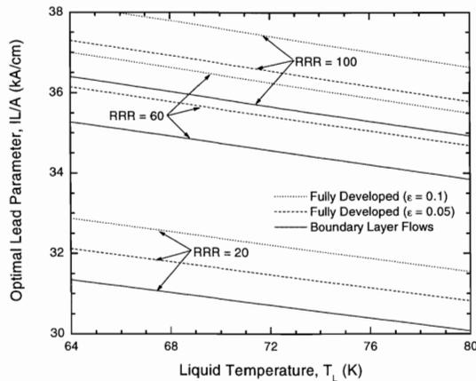
**FIGURE 4.** Optimal lead parameter as a function of liquid temperature with various RRR values of copper for boundary layer flow and fully developed flow.
